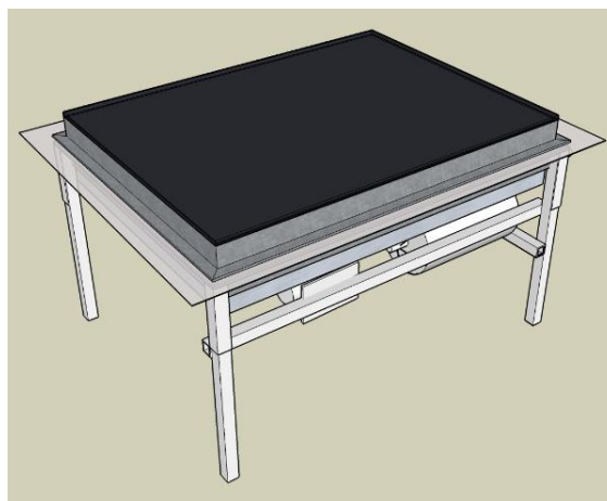
Fig. 5: Sketch of the test apparatus with the clamped membrane and inserted panel which is joined to the membrane with adhesive tape (yellow) (left). Test apparatus sealed with the cover panel for determining the test stand leakage (right).
