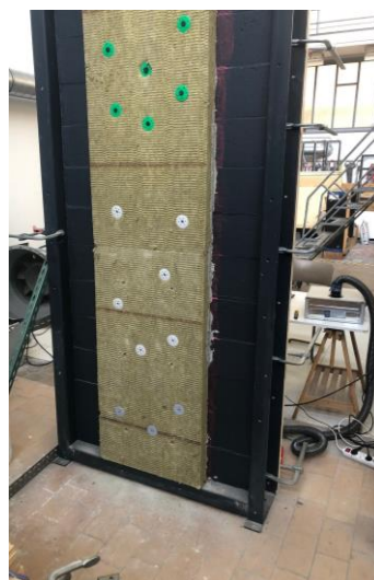
Figures 14: Concrete walls with BLOWERPROOF® LIQUID (left) and ISOPROOF FR (right), PRIMER 52, REDArt™ CAPA BASE CASA, ROCKWOOL® ROCKSATE DUO PLUS and 15 anchors (6 green Ejot H2, 6 white Ejot STR U 2G, 3 grey Rawlplug®)
