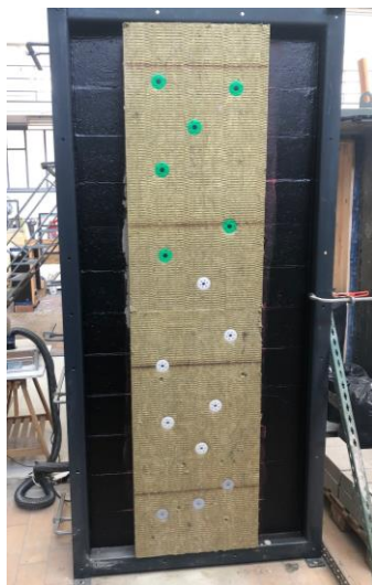
Figures 14: Concrete walls with BLOWERPROOF® LIQUID (left) and ISOPROOF FR (right), PRIMER 52, REDArt™ CAPA BASE CASA, ROCKWOOL® ROCKSATE DUO PLUS and 15 anchors (6 green Ejot H2, 6 white Ejot STR U 2G, 3 grey Rawlplug®)
