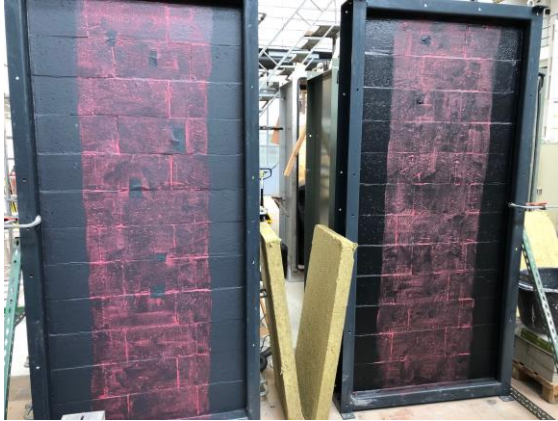
Figure 7: PRIMER 52 was applied with brush
