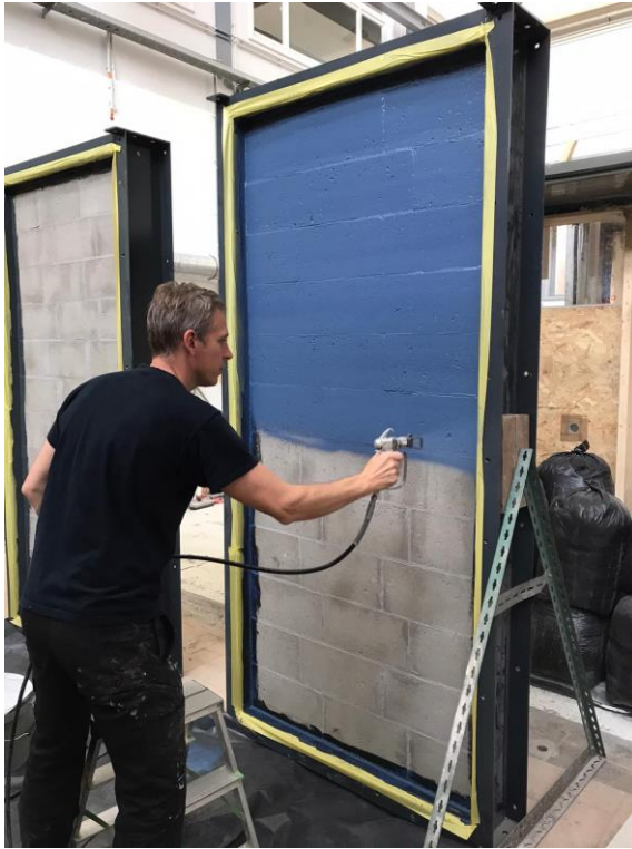
Figures 2: Airless application of BLOWERPROOF® LIQUID (left) and ISOPROOF FR (right)
