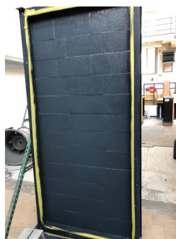
Figures 3: Walls covered with BLOWERPROOF® LIQUID (left) and ISOPROOF FR (right)
